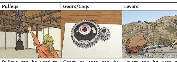
Pulleys can be used to make a small force lift a lighter load. The more wheels in a pulley, the less force is needed to lift a weight.
